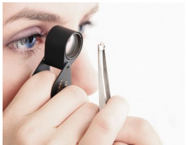
Diamond Grading Lab students assess a diamond's clarity using a 10X jeweller's loupe - ©GIA
